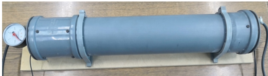
Fig. 3. Ozonizer for disinfection of beehives
